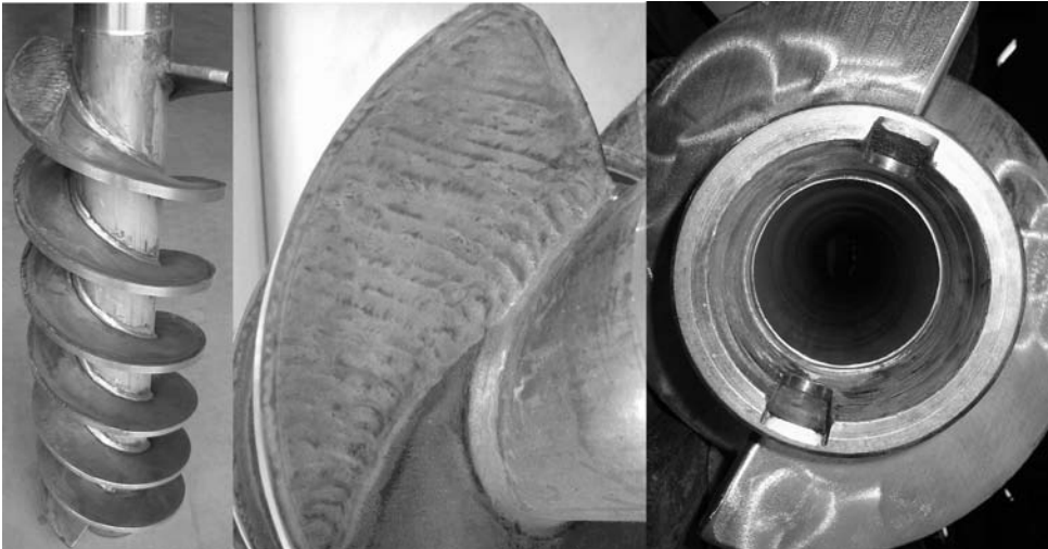
picture 4.9: Auger with re-enforced flight and hub connection, new condition
