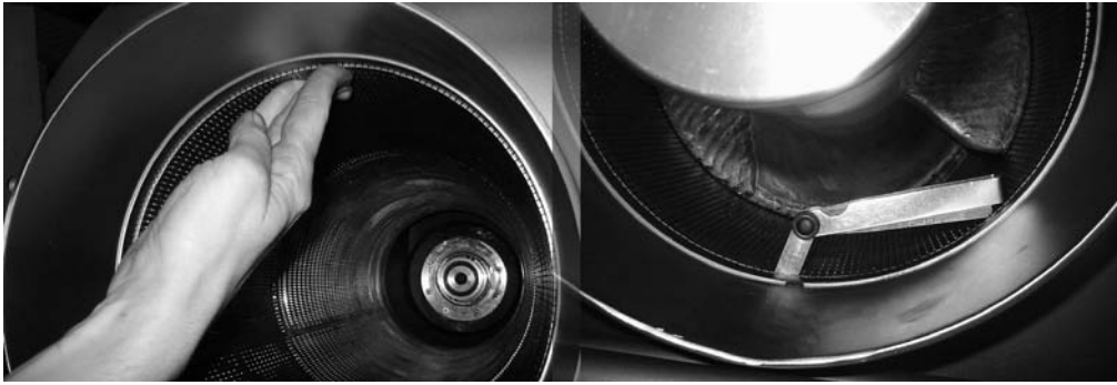
picture 4.8: Movable screen in the Separator checked by hand (left side) and checked with a feeler gauge (right side)
