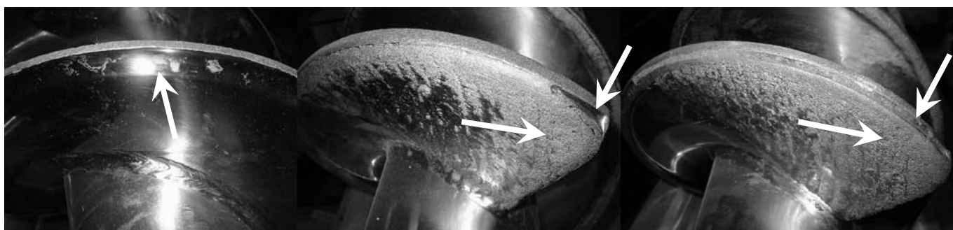
picture. 4.13: Indications for the necessity of the auger refurbishment
